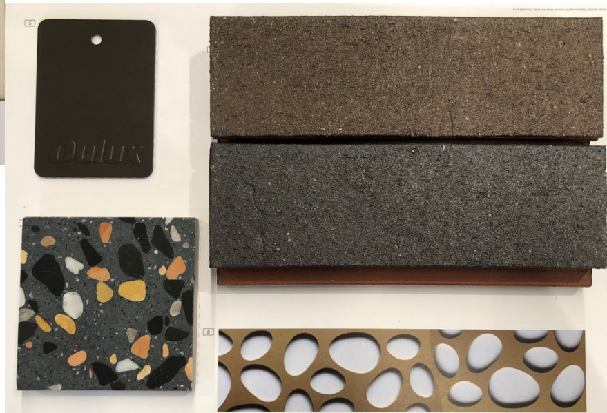
1. FORMED LIGHT TINTED CONCRETE W/ BOLT HOLES 2. PGH BRICK MORADA BLANCO SPLITS 3. PGH BRICK MORADA NERO SPLITS 4. METAL FENCES, BALUSTRADES (GF, L1 & L2) & FACADE METAL EDGES & TRIMS, DULUX DURATEC NATURAL BRONZE POWDERCOAT 5. METAL AWNINGS, STEEL BEAMS & COLUMNS, DULUX ELECTRO DARK BRONZE POWDERCOAT
